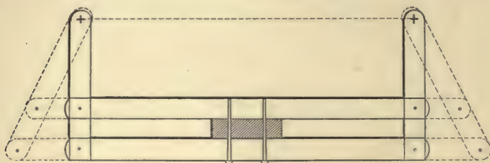
FIG. 7.—COLBY'S MEASURING ROD.
